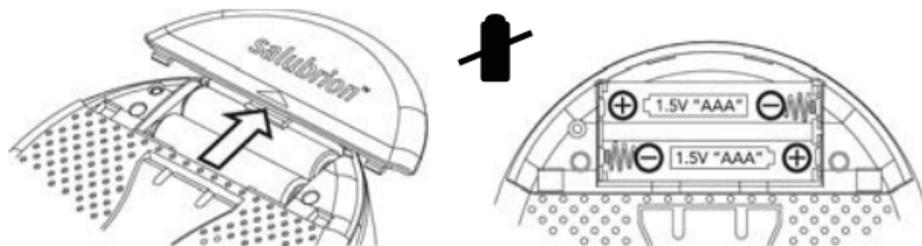
Low battery power can cause the Enso Clock to malfunction. Symptoms may include the clock display freezing, the buttons not responding to input, random resetting, or degradation in audio quality. These problems can usually be remedied by a fresh set of batteries.
